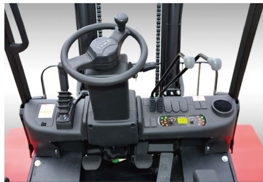
Ergonomic instrument panel: integrated handle switch, ratchet type hand brake and integrated electro-hydraulic reversing handle
