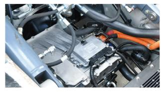
The integrated power system reduces the wiring harness which greatly reduces the loss of electric energy transmission. And the levels of parts and control modules are clear and convenient for maintenance;
