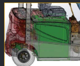
Middle and sink layout of the battery
