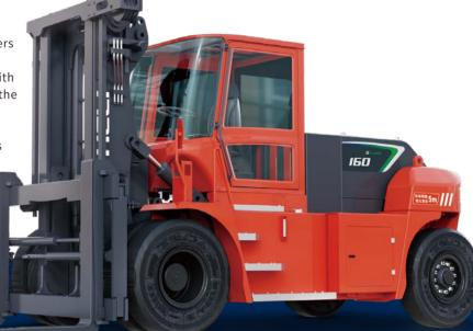
The truck is equipped with potential energy recovery and kinetic energy regenerative energy technology, thorugh
